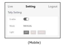
Tally has two modes, manual and automatic mode. After the tally light is set successfully, the color of the camera icon in the upper right corner of the web page will also change with the tally light.
