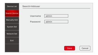
(2) Press the MENU button to enter the menu and select to manually add the camera IP, port, user name, password, and select the Onvif protocol point to save (the camera and keyboard must be on the same network segment)
