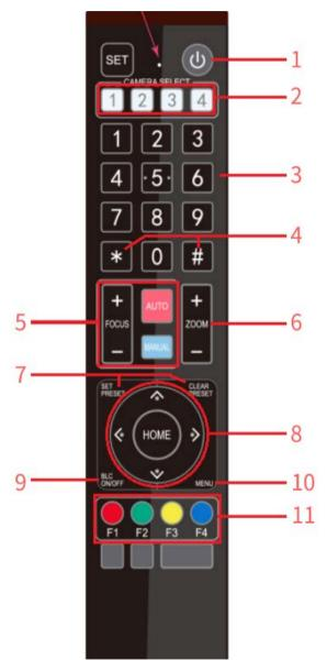
Finishing initialization, it can receive and execute the IR commands. Press the remote controller button, the indicator light is flashing; release the button, the indicator light stops flashing. Users can control the pan/tilt/zoom, setting and running preset positions via remote controller.
