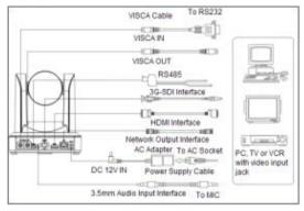
Figure 2.5.1 PTZ model external interface diagram
