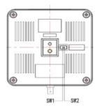
Figure 2.5.2 Bottom Dial Switch diagram PTZ model: two DIP switches are set to ON or OFF to select different modes of operation as shown in Table 2.5.2.
