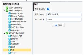
Login on the web page by NEW camera IP address, and check NDI Enable to enable the NDI.
